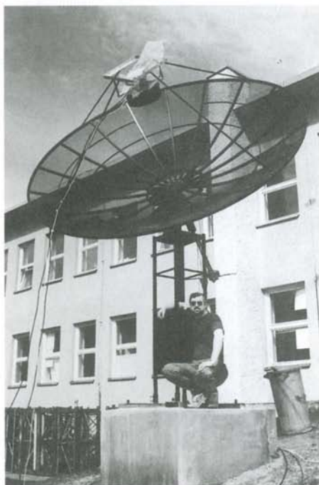
OK1DFC 3.8m Dish for 1296 with VE4MA feed
